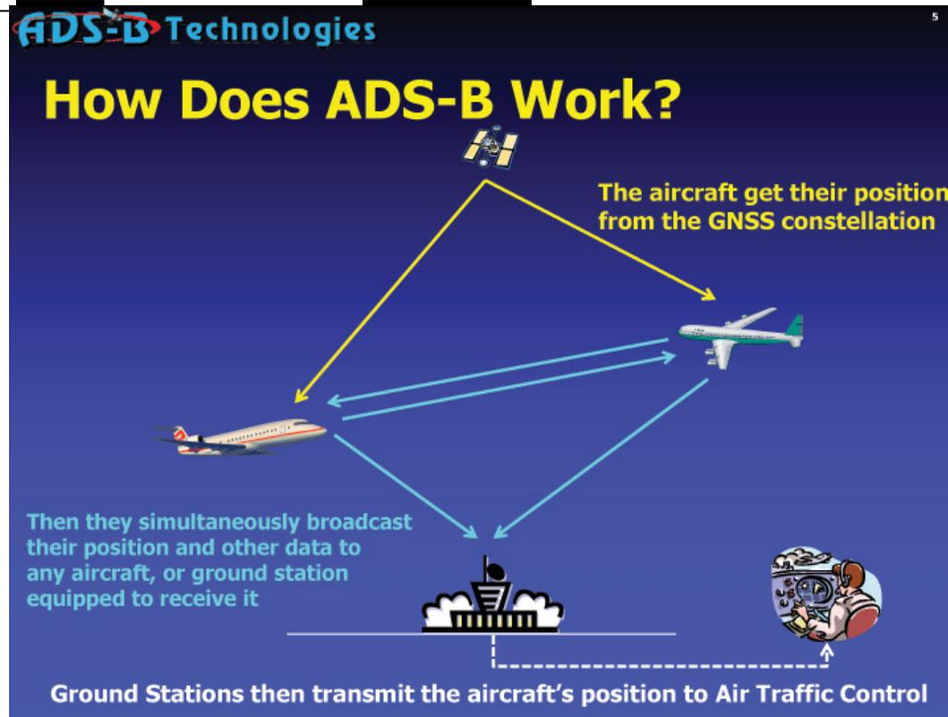
ADS-B enables broadcast of identification, position, altitude and speed to aircraft and ATC. This is **ADS-B OUT** services. Mandatory equipment compliance by 2020.
