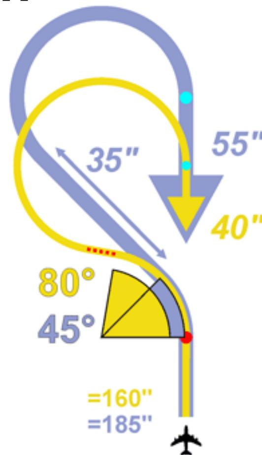
A procedure turn will get the plane back on the inbound course. Turn left to a heading of  $012^{\circ}$ , and fly for a minute (more or less, depending on wind). Then, make a standard rate turn to the right, completely around to a heading of  $192^{\circ}$ . Twist the OBS to  $237$ . As the CDI centers, turn inbound to track the  $237^{\circ}$  TO course.
