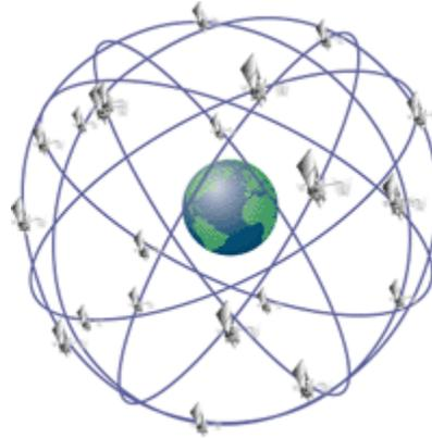
The Global Positioning System (GPS) is a space-based radio-navigation system consisting of a constellation of satellites and a network of ground stations used for monitoring and control. Currently 32 GPS satellites orbit the Earth at an altitude of approximately 11,000 miles providing users with accurate information on position, velocity, and time anywhere in the world and in all weather conditions.
